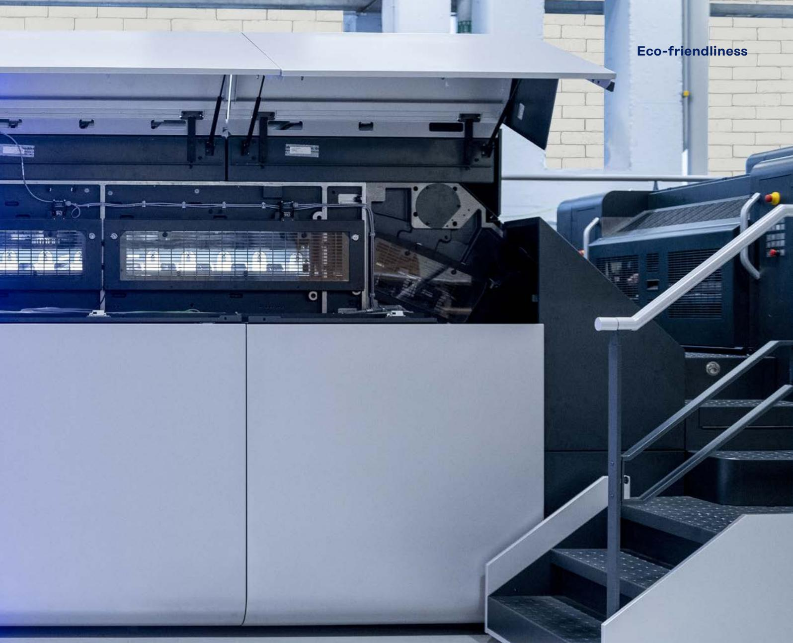
It starts with the VariDry dryer family: The **VariDry<sup>Blue</sup>** IR/TL dryers in delivery and delivery extension combine maximum drying performance with low energy consumption. By reusing the recirculated air as drying air, we reduce the energy requirements compared with conventional dryers several times over. This has an impact on the entire printing process, as drying usually involves the highest electricity consumption.
